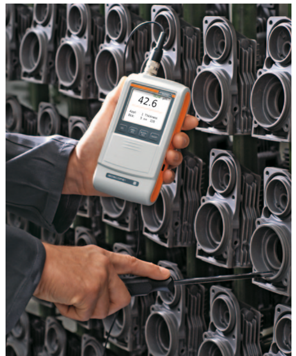
Measurements using the internal probe FAI 3.3-150
